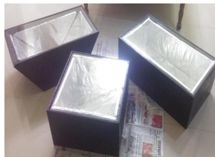
Fig.1 Fabricated Geometrical Shapes of Box Type Solar Cooker
